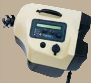
Blue Ox's Patriot proportional portable braking system has an LED display and one setup button. The unit is controlled by an in-coach wireless module. The Patriot has a built-in battery and utilizes an electric cylinder to activate braking arm.
