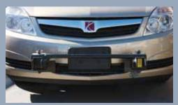
Once the proper baseplate is installed, this clean-looking setup is all that remains when the towed vehicle isn't hooked up; cooling doesn't suffer.
