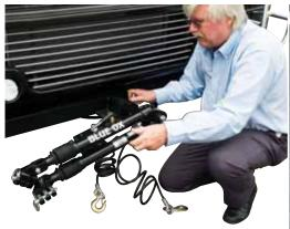
Once the tow bar is attached to both vehicles, make sure electric connections and safety cables are secure.
