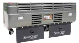
Adding large rubber flaps at the rear of a motorhome will minimize towed-vehicle damage from debris, dirt and grime kicked up by coach tires.
